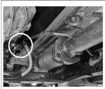
1. Locate factory exhaust pressure sensor.
